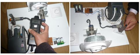
Fig. 6. Determination of the operating parameters of the magnetic sensors
