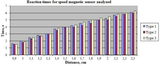
Fig. 8. Sensor reaction times depending on distance and rotational speed
