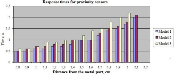
Fig. 7. Correlation of reaction times of proximity sensors with the distance to the landmark
