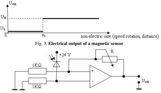
Fig. 4. Electronic circuit used to obtain the output size  $(U_{out})$
