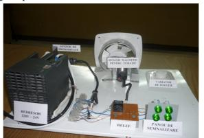
Fig. 5. Electronic assembly used to study the operation of the two types of magnetic sensors
